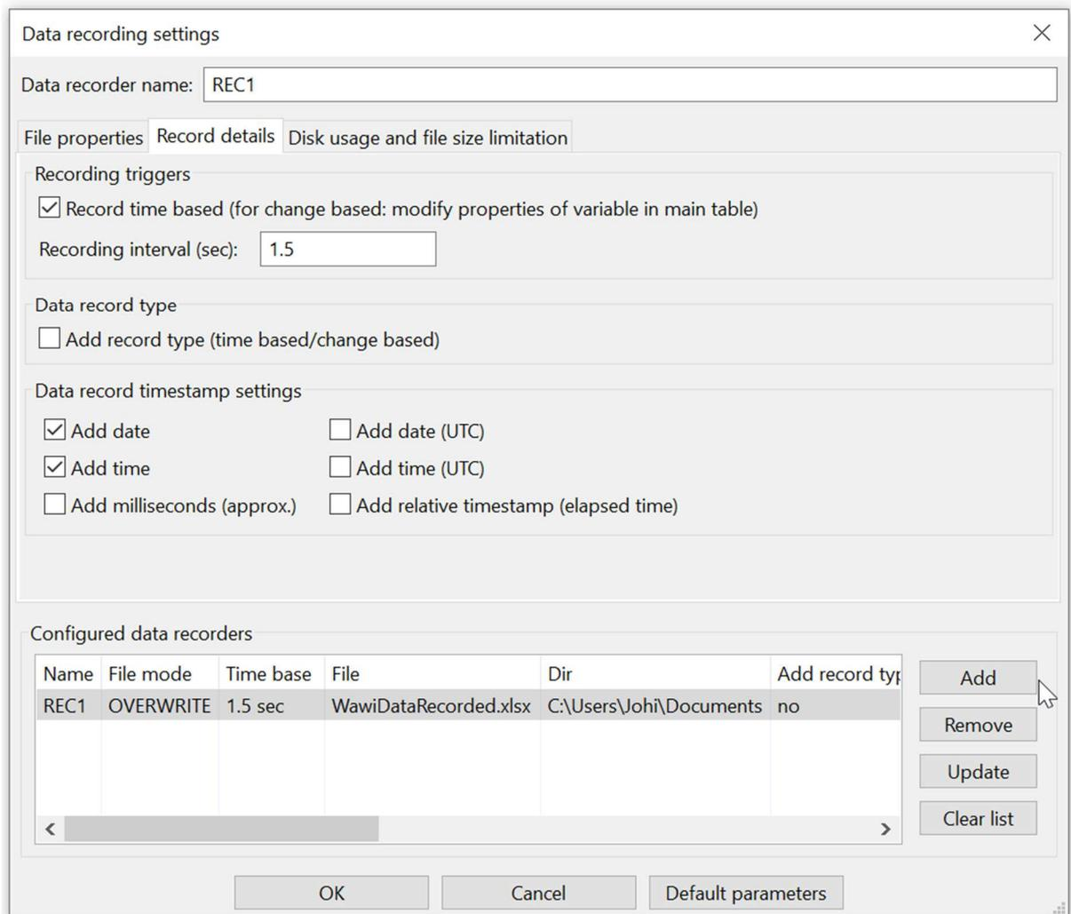
Fig. 8.2. The data recorder setup dialog, timing = 1.5 sec.
