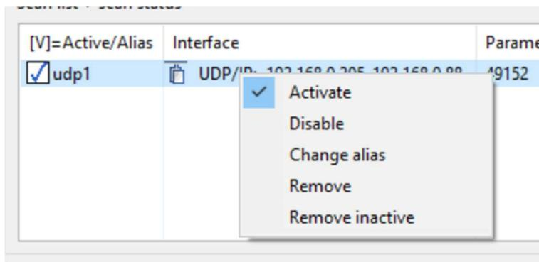
Fig. 6.4. Modify the status of a connection without or after scanning.
