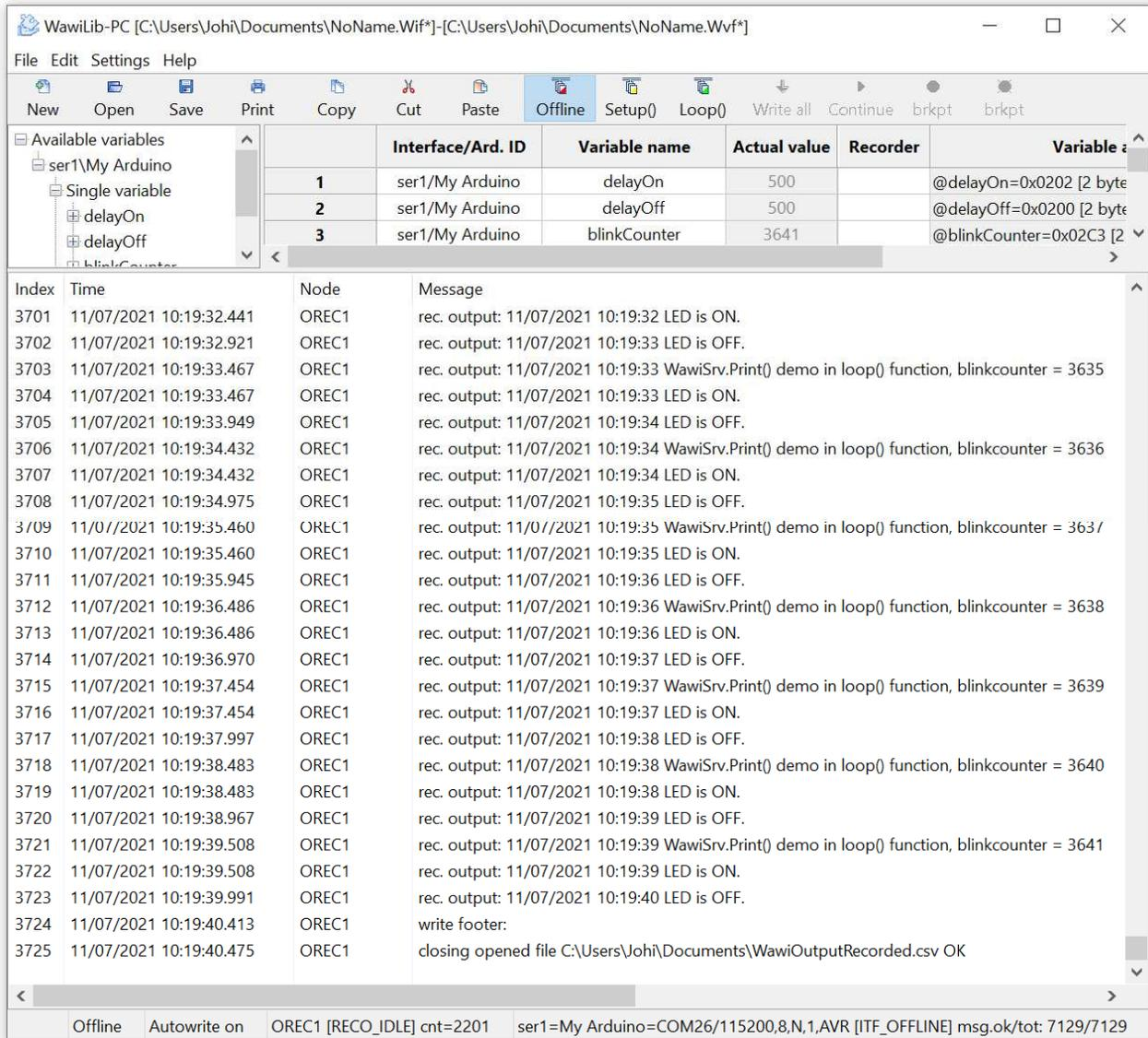
fig 9.5. Arduino output recording displayed in window.
