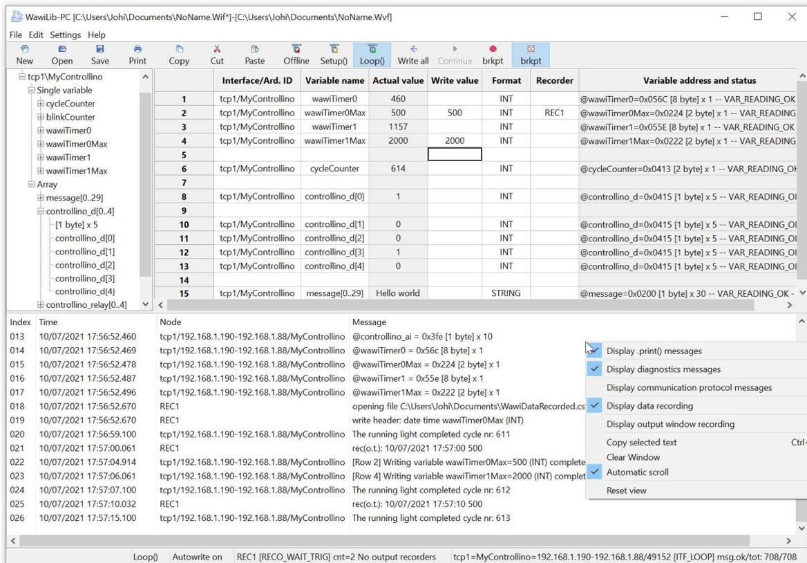
fig 5.4. WawiLib overview in a Controllino TCP configuration.
