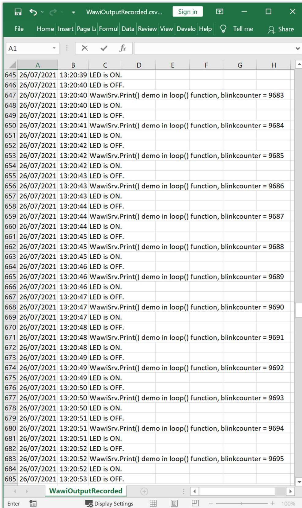
fig 9.6. Arduino output recording file opened in Excel.
