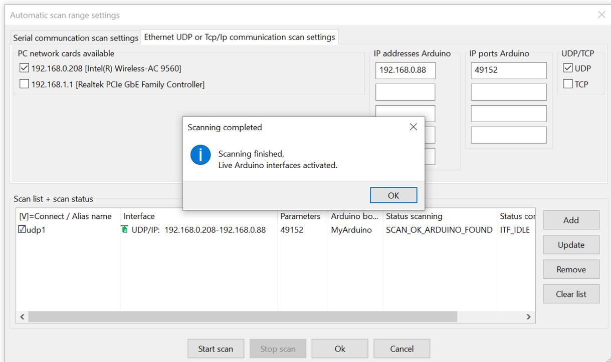
Fig. 6.3. Ethernet communication setup indicating successful link check.
