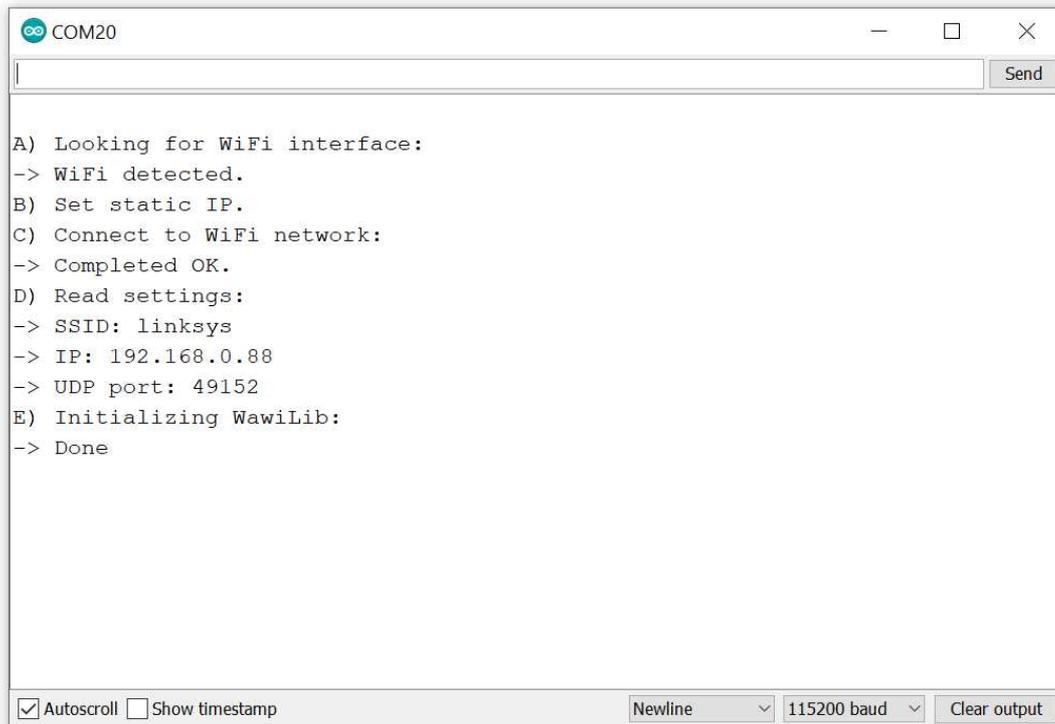
Fig. 4.7. Serial monitor output indicating an proper initialization of WawiLib in the Sketch.
