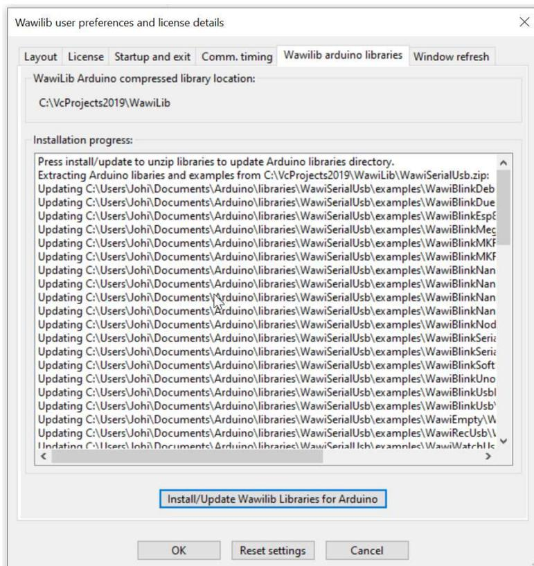
Fig. 2.3. Manual install of Arduino libraries.
