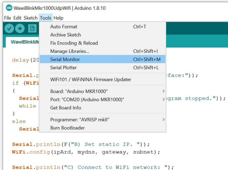
Fig. 4.6. Open the serial monitor window.
