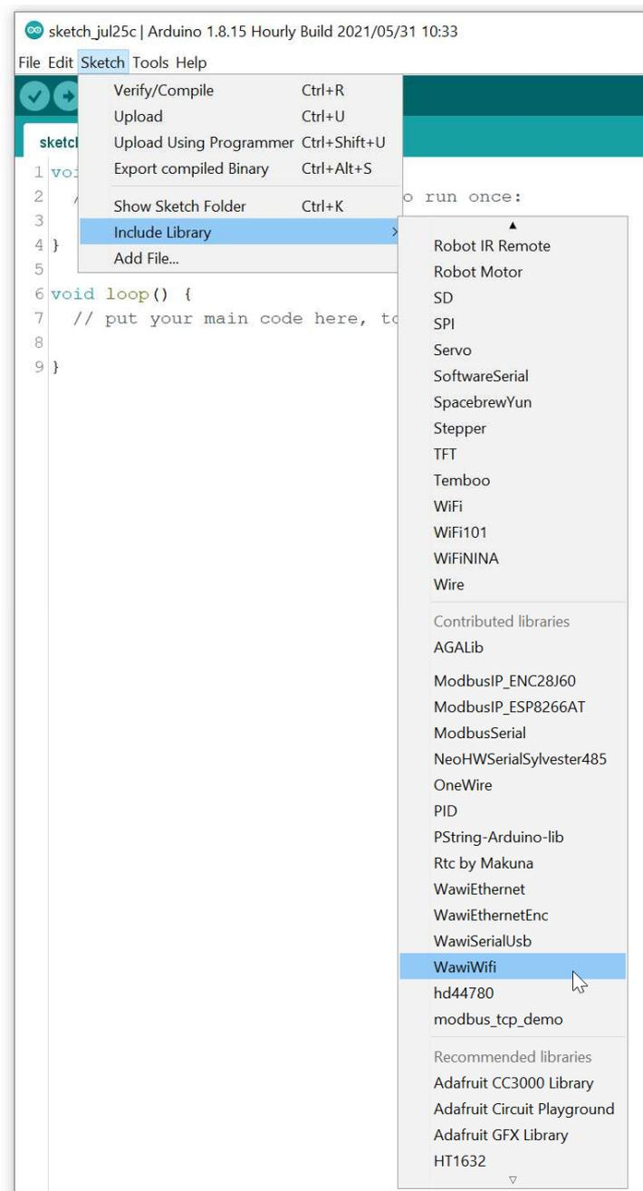
Fig. 2.1. Check the installation WawiWifi library in the Arduino IDE.
