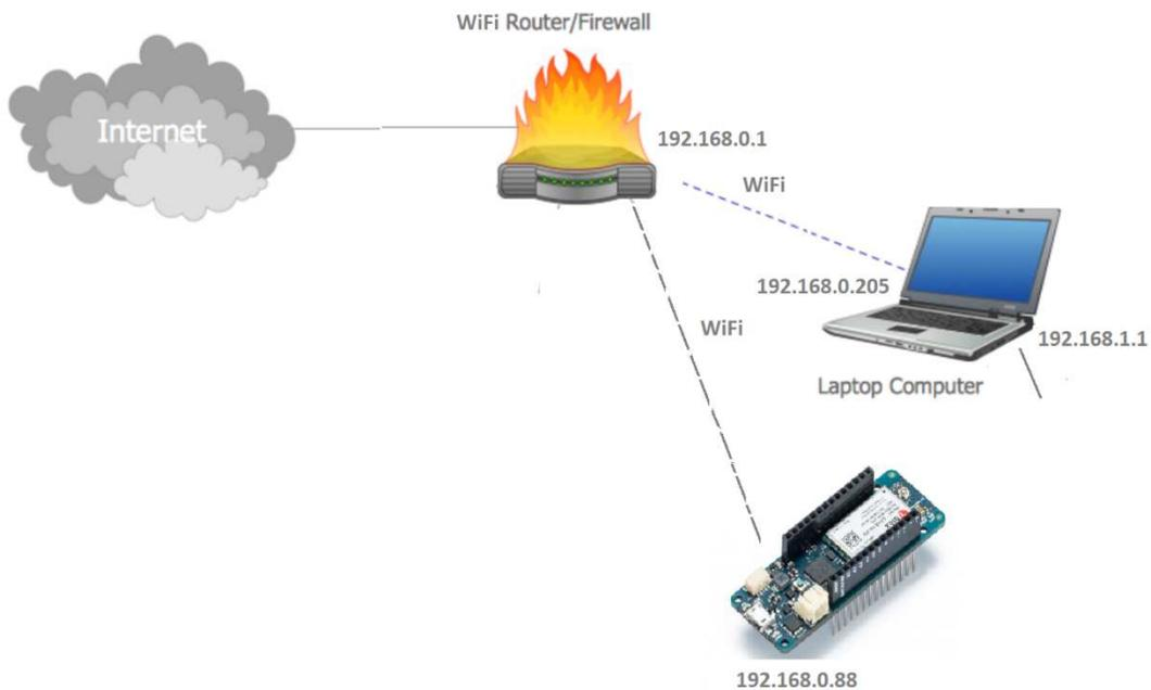
Fig. 3.1. Test network architecture overview.
